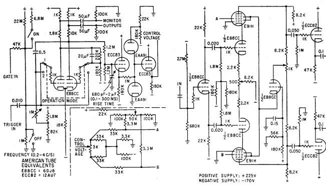
DRIVER FOR FADER—Can be operated either in free-running mode or in triggered or gated mode, to produce control voltage that will drive electronic fader. Correction network at lower right transfers control voltage to fader and minimizes switching transient.
