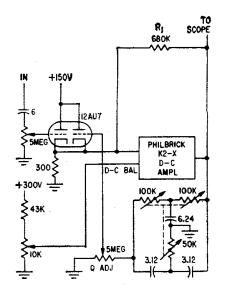
TUNABLE SUBAUDIO AMPLIFIER—Commercial d-c amplifier with twin-T feedback tuning element tunes from 0.5 to 100 cps, for analyzing low-frequency components of complex waveforms.
